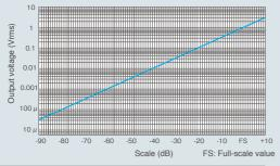
Output voltage: 1 Vrms ±50 mVrms (scale upper limit)
